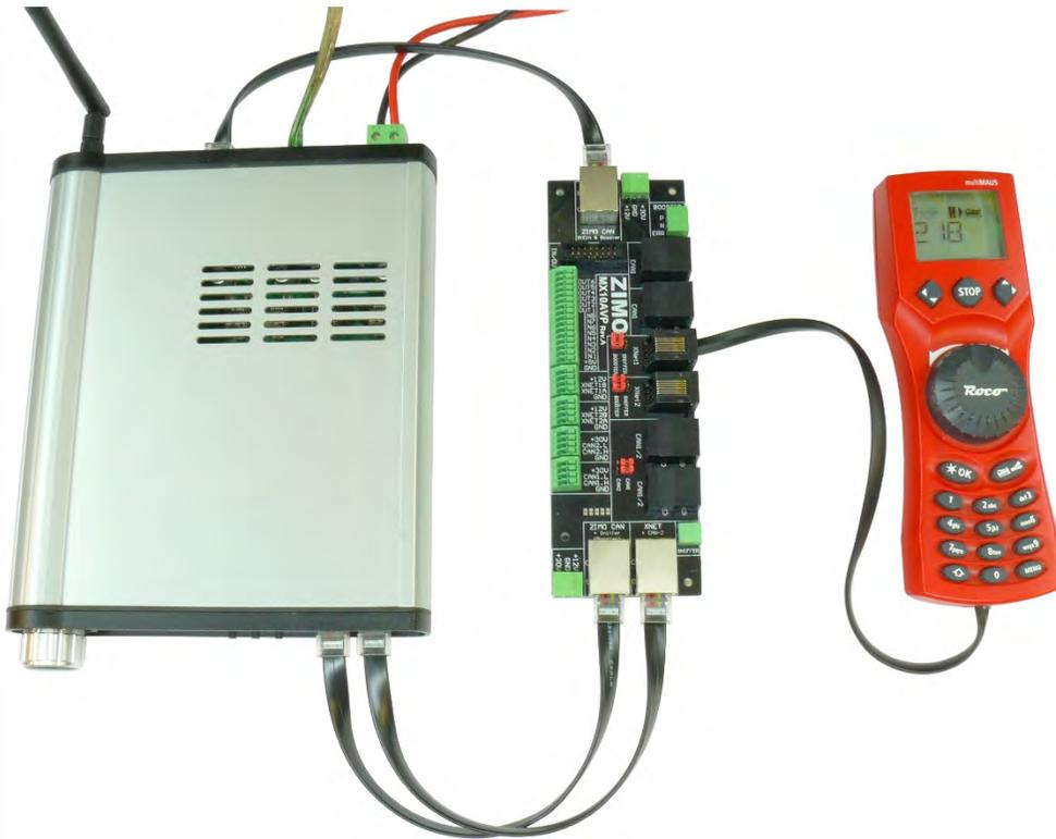
*Connecting a Roco Multimaus via a 6-pole cable to an XNET socket on the MX10AVP.
