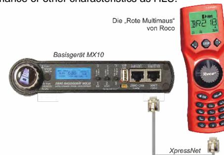
The wired (red) *multiMAUS* is connected via a corresponding cable to the XNET socket of the MX10 (front side). In the menu "Bus Config+Monitor", under "XNET1" change to "for Lokmouse".
