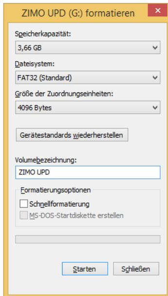
As shown in the window on the left, the flash drive has to be formatted in the filesystem **FAT32** to update the MX10. The Cluster size shall be set to **4096 Bytes** (= 4kB).
