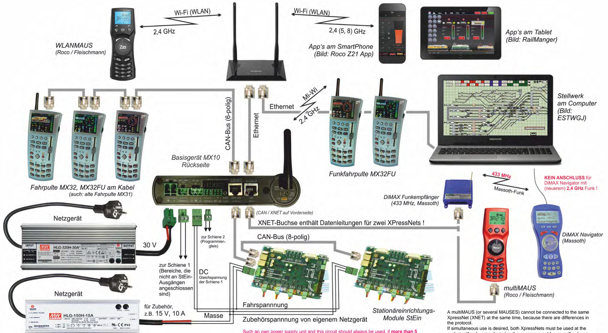
Such an own power supply unit and this circuit should always be used, if more than 5 StEin modules (with MX10) or more than 1 StEin module (with MX10EC) are used. Only in smaller applications is it advisable to use the accessory voltage for the StEin (which also covers the internal consumption of the modules) from the "DC-out" output S2 of the MX10 or 12 V of the MX10EC.
